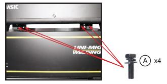
Line up brackets and tighten into place using 4 x A screws.
